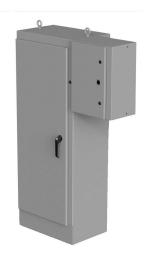
Saginaw enclosure, NEMA 3R/12/13, 84 x 40 x 18in (HxWxD), freestanding, carbon steel, ANSI 61 gray, powder coat finish, single-door, 3-point padlocking handle, subpanel and external rotary disconnect enclosure included.
