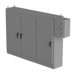
Saginaw enclosure, NEMA 3R/12/13, 84 x 118 x 18in (HxWxD), freestanding, carbon steel, ANSI 61 gray, powder coat finish, 3-door, 3-point padlocking handle, external rotary disconnect enclosure included.
