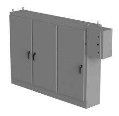
Saginaw enclosure, NEMA 3R/12/13, 84 x 118 x 18in (HxWxD), freestanding, carbon steel, ANSI 61 gray, powder coat finish, 3-door, 3-point padlocking handle, subpanel and external rotary disconnect enclosure included.
