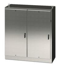
Saginaw disconnect enclosure, NEMA 3R/4/4X/12/13, right flange, 84 x 78 x 24in (HxWxD), freestanding, 304 stainless steel, #4 brush finish, 2-door, 3-point padlocking handle, powder coated subpanel included.
