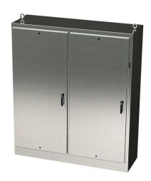
Saginaw disconnect enclosure, NEMA 3R/4/4X/12/13, right flange, 84 x 78 x 24in (HxWxD), freestanding, 316L stainless steel, #4 brush finish, 2-door, 3-point padlocking handle, powder coated subpanel included.
