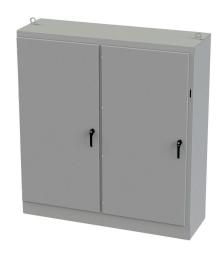
Saginaw disconnect enclosure, NEMA 3R/12/13, right flange, 84 x 78 x 24in (HxWxD), freestanding, carbon steel, ANSI 61 gray, powder coat finish, 2-door, 3-point padlocking handle, galvanized subpanel included.
