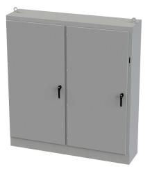
Saginaw disconnect enclosure, NEMA 3R/12/13, right flange, 84 x 78 x 18in (HxWxD), freestanding, carbon steel, ANSI 61 gray, powder coat finish, 2-door, 3-point padlocking handle, powder coated subpanel included.
