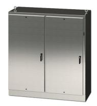
Saginaw disconnect enclosure, NEMA 3R/4/4X/12/13, right flange, 84 x 78 x 18in (HxWxD), freestanding, 304 stainless steel, #4 brush finish, 2-door, 3-point padlocking handle, powder coated subpanel included.
