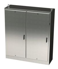
Saginaw disconnect enclosure, NEMA 3R/4/4X/12/13, right flange, 84 x 78 x 18in (HxWxD), freestanding, 316L stainless steel, #4 brush finish, 2-door, 3-point padlocking handle, powder coated subpanel included.
