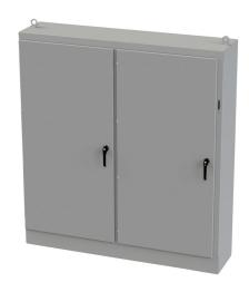
Saginaw disconnect enclosure, NEMA 3R/12/13, right flange, 84 x 78 x 18in (HxWxD), freestanding, carbon steel, ANSI 61 gray, powder coat finish, 2-door, 3-point padlocking handle, galvanized subpanel included.
