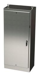
Saginaw disconnect enclosure, NEMA 3R/4/4X/12/13, right flange, 84 x 40 x 24in (HxWxD), freestanding, 316L stainless steel, #4 brush finish, single-door, 3-point padlocking handle, powder coated subpanel included.
