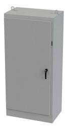
Saginaw disconnect enclosure, NEMA 3R/12/13, right flange, 84 x 40 x 24in (HxWxD), freestanding, carbon steel, ANSI 61 gray, powder coat finish, single-door, 3-point padlocking handle, galvanized subpanel included.
