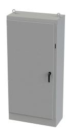
Saginaw disconnect enclosure, NEMA 3R/12/13, right flange,  $84 \times 40 \times 18$  in (HxWxD), freestanding, carbon steel, ANSI 61 gray, powder coat finish, single-door, 3-point padlocking handle, powder coated subpanel included.
