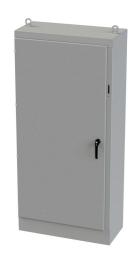
Saginaw disconnect enclosure, NEMA 3R/12/13, right flange,  $84 \times 40 \times 18$  in (HxWxD), freestanding, carbon steel, ANSI 61 gray, powder coat finish, single-door, 3-point padlocking handle, galvanized subpanel included.
