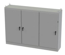
Saginaw disconnect enclosure, NEMA 3R/12/13, right flange, 84 x 118 x 24in (HxWxD), freestanding, carbon steel, ANSI 61 gray, powder coat finish, 3-door, 3-point padlocking handle, (2) powder coated subpanels included.
