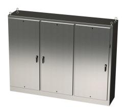
Saginaw disconnect enclosure, NEMA 3R/4/4X/12/13, right flange, 84 x 118 x 24in (HxWxD), freestanding, 316L stainless steel, #4 brush finish, 3-door, 3-point padlocking handle, (2) powder coated subpanels included.
