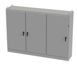
Saginaw disconnect enclosure, NEMA 3R/12/13, right flange, 84 x 118 x 24in (HxWxD), freestanding, carbon steel, ANSI 61 gray, powder coat finish, 3-door, 3-point padlocking handle, (2) galvanized subpanels included.
