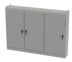
Saginaw disconnect enclosure, NEMA 3R/12/13, right flange, 84 x 118 x 18in (HxWxD), freestanding, carbon steel, ANSI 61 gray, powder coat finish, 3-door, 3-point padlocking handle, (2) powder coated subpanels included.
