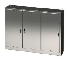
Saginaw disconnect enclosure, NEMA 3R/4/4X/12/13, right flange, 84 x 118 x 18in (HxWxD), freestanding, 304 stainless steel, #4 brush finish, 3-door, 3-point padlocking handle, (2) powder coated subpanels included.
