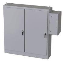
Saginaw enclosure, NEMA 3R/12/13, 84 x 78 x 18in (HxWxD), freestanding, carbon steel, ANSI 61 gray, powder coat finish, 2-door, 3-point padlocking handle, external disconnect enclosure included.
