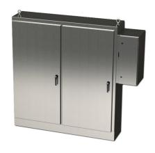
Saginaw enclosure, NEMA 3R/4/4X/12/13, 84 x 78 x 18in (HxWxD), freestanding, 304 stainless steel, #4 brush finish, 2-door, 3-point padlocking handle, external disconnect enclosure included.
