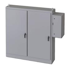
Saginaw enclosure, NEMA 3R/12/13, 84 x 78 x 18in (HxWxD), freestanding, carbon steel, ANSI 61 gray, powder coat finish, 2-door, 3-point padlocking handle, subpanel and external disconnect enclosure included.
