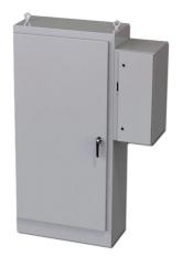
Saginaw enclosure, NEMA 3R/12/13, 84 x 40 x 18in (HxWxD), freestanding, carbon steel, ANSI 61 gray, powder coat finish, single-door, 3-point padlocking handle, external disconnect enclosure included.
