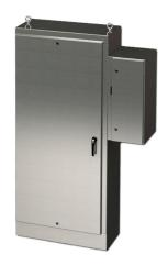
Saginaw enclosure, NEMA 3R/4/4X/12/13, 84 x 40 x 18in (HxWxD), freestanding, 316L stainless steel, #4 brush finish, single-door, 3-point padlocking handle, external disconnect enclosure included.
