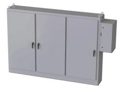
Saginaw enclosure, NEMA 3R/12/13, 84 x 118 x 18in (HxWxD), freestanding, carbon steel, ANSI 61 gray, powder coat finish, 3-door, 3-point padlocking handle, external disconnect enclosure included.
