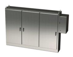
Saginaw enclosure, NEMA 3R/4/4X/12/13, 84 x 118 x 18in (HxWxD), freestanding, 304 stainless steel, #4 brush finish, 3-door, 3-point padlocking handle, external disconnect enclosure included.
