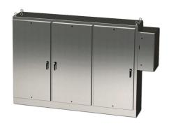
Saginaw enclosure, NEMA 3R/4/4X/12/13, 84 x 118 x 18in (HxWxD), freestanding, 316L stainless steel, #4 brush finish, 3-door, 3-point padlocking handle, external disconnect enclosure included.
