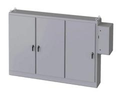
Saginaw enclosure, NEMA 3R/12/13, 84 x 118 x 18in (HxWxD), freestanding, carbon steel, ANSI 61 gray, powder coat finish, 3-door, 3-point padlocking handle, subpanel and external disconnect enclosure included.
