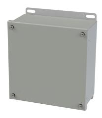
Saginaw enclosure, NEMA 3R/4/12/13, 8 x 8 x 4in (HxWxD), wall mount, carbon steel, ANSI 61 gray, powder coat finish, screw cover.
