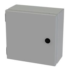
Saginaw Enviroline Junction series enclosure, NEMA 3R/4/12/13, 8 x 8 x 4in (HxWxD), wall mount, carbon steel, ANSI 61 gray, powder coat finish, single-door, 1/4-turn semi-flush latch.
