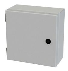
Saginaw Enviroline Junction series enclosure, NEMA 3R/4/12/13, 8 x 8 x 4in (HxWxD), wall mount, carbon steel, RAL 7035 light gray, powder coat finish, single-door, 1/4-turn semi-flush latch.
