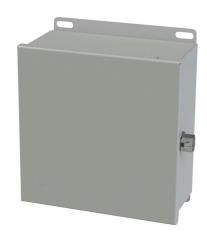
Saginaw enclosure, NEMA 3R/4/12/13,  $8 \times 8 \times 4$  in (HxWxD), wall mount, carbon steel, ANSI 61 gray, powder coat finish, singledoor, stainless steel clamps.
