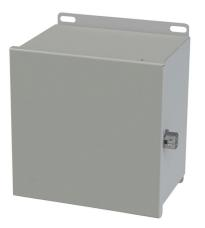
Saginaw enclosure, NEMA 3R/4/12/13, 8 x 8 x 6in (HxWxD), wall mount, carbon steel, ANSI 61 gray, powder coat finish, single-door, stainless steel clamps.
