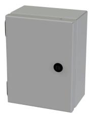
Saginaw Enviroline Junction series enclosure, NEMA 3R/4/12/13, 8 x 6 x 4in (HxWxD), wall mount, carbon steel, ANSI 61 gray, powder coat finish, single-door, 1/4-turn semi-flush latch.
