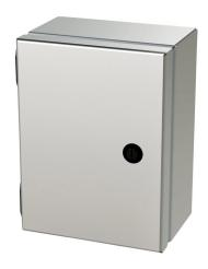
Saginaw Enviroline Junction series enclosure, NEMA 3R/4/4X/12/13, 8 x 6 x 4in (HxWxD), wall mount, 304 stainless steel, #4 brush finish, single-door, 1/4-turn semi-flush latch.
