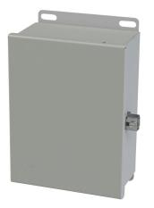
Saginaw enclosure, NEMA 3R/4/12/13, 8 x 6 x 3.5in (HxWxD), wall mount, carbon steel, ANSI 61 gray, powder coat finish, single-door, stainless steel clamps.
