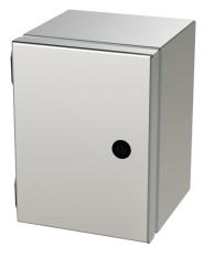
Saginaw Enviroline Junction series enclosure, NEMA 3R/4/4X/12/13, 8 x 6 x 6in (HxWxD), wall mount, 304 stainless steel, #4 brush finish, single-door, 1/4-turn semi-flush latch.
