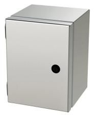
Saginaw Enviroline Junction series enclosure, NEMA 3R/4/4X/12/13, 8 x 6 x 6in (HxWxD), wall mount, 316L stainless steel, #4 brush finish, single-door, 1/4-turn semi-flush latch.
