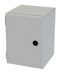
Saginaw Enviroline Junction series enclosure, NEMA 3R/4/12/13, 8 x 6 x 6in (HxWxD), wall mount, carbon steel, RAL 7035 light gray, powder coat finish, single-door, 1/4-turn semi-flush latch.
