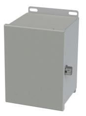
Saginaw enclosure, NEMA 3R/4/12/13, 8 x 6 x 6in (HxWxD), wall mount, carbon steel, ANSI 61 gray, powder coat finish, single-door, stainless steel clamps.
