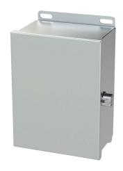
Saginaw enclosure, NEMA 3R/4/4X/12/13, 8 x 6 x 4in (HxWxD), wall mount, 316L stainless steel, #4 brush finish, single-door, stainless steel clamps.
