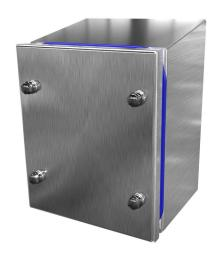
Saginaw sanitary enclosure, slope top, NEMA 3R/4/4X/12, 7 x 6 x 4in (HxWxD), wall mount, 304 stainless steel, #4 brush finish, screw cover.
