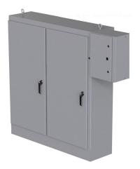
Saginaw enclosure, NEMA 3R/12/13, 72 x 78 x 18in (HxWxD), freestanding, carbon steel, ANSI 61 gray, powder coat finish, 2-door, 3-point padlocking handle, external rotary disconnect enclosure included.
