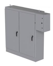
Saginaw enclosure, NEMA 3R/12/13, 72 x 66 x 18in (HxWxD), freestanding, carbon steel, ANSI 61 gray, powder coat finish, 2-door, 3-point padlocking handle, subpanel and external rotary disconnect enclosure included.
