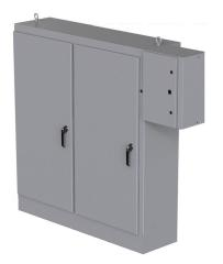
Saginaw enclosure, NEMA 3R/4/12/13, 72 x 54 x 18in (HxWxD), freestanding, carbon steel, ANSI 61 gray, powder coat finish, 2-door, 3-point padlocking handle, subpanel and external rotary disconnect enclosure included.
