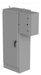
Saginaw enclosure, NEMA 3R/12/13, 72 x 40 x 18in (HxWxD), freestanding, carbon steel, ANSI 61 gray, powder coat finish, single-door, 3-point padlocking handle, subpanel and external rotary disconnect enclosure included.
