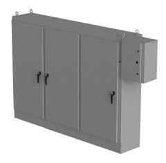
Saginaw enclosure, NEMA 3R/12/13, 72 x 118 x 18in (HxWxD), freestanding, carbon steel, ANSI 61 gray, powder coat finish, 3-door, 3-point padlocking handle, external rotary disconnect enclosure included.
