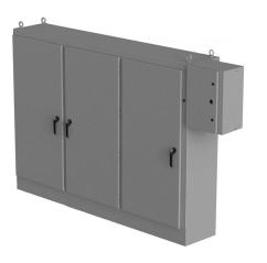
Saginaw enclosure, NEMA 3R/12/13, 72 x 118 x 18in (HxWxD), freestanding, carbon steel, ANSI 61 gray, powder coat finish, 3-door, 3-point padlocking handle, subpanel and external rotary disconnect enclosure included.
