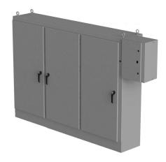
Saginaw enclosure, NEMA 3R/12/13, 72 x 100 x 18in (HxWxD), freestanding, carbon steel, ANSI 61 gray, powder coat finish, 3-door, 3-point padlocking handle, external rotary disconnect enclosure included.
