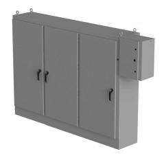
Saginaw enclosure, NEMA 3R/12/13, 72 x 100 x 18in (HxWxD), freestanding, carbon steel, ANSI 61 gray, powder coat finish, 3-door, 3-point padlocking handle, subpanel and external rotary disconnect enclosure included.
