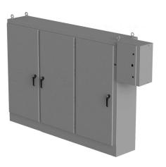
Saginaw enclosure, NEMA 3R/12/13, 72 x 100 x 18in (HxWxD), freestanding, carbon steel, ANSI 61 gray, powder coat finish, 3-door, 3-point padlocking handle, subpanel and external rotary disconnect enclosure included.
